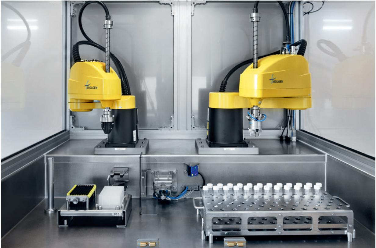
**High throughput:** the PurePrep TTR system fully automatically prepares 320 patient samples per hour for PCR testing.
