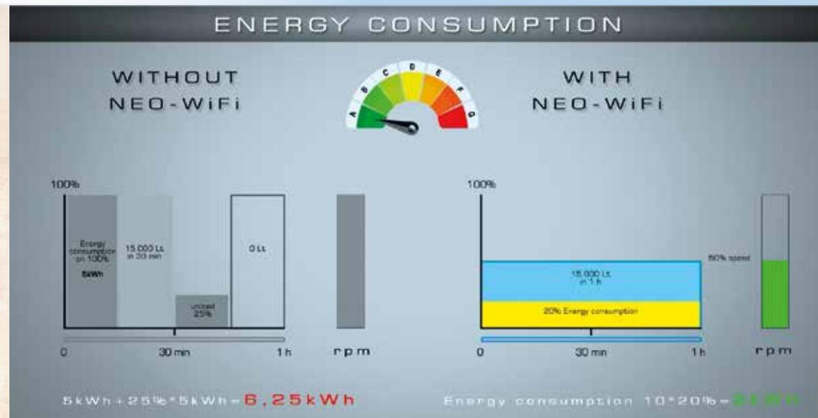
$$\frac{kW1}{kW2} = \frac{rpm1^3}{rpm2^3}$$
